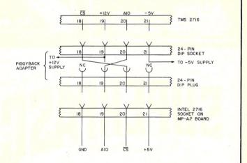
Fig. 2. Alternate method for + 12 V and - 5 V supplies to TMS 2716 EPROMs. This leaves the MP-A2 board intact.
